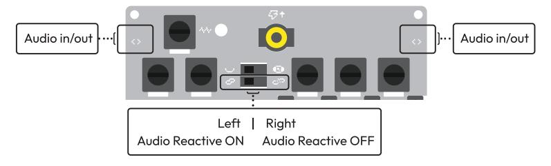
Simply audio signal can be connected to input on the Left to the Right output of the socket or vice-versa.
